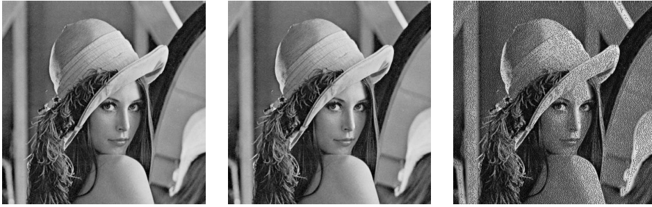
FIG. 1. Lossy compression of “Lena” at 1/3 ‘o’/char density yields a gain of 25,33% over GZip. Interpolation (center figure) leaves 10,13% differences from original, unnoticeable to the naked eye.
